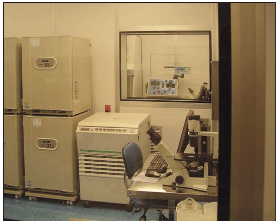
FIGURE 4. View of cleanroom #2. Cleanroom #1 is visible through the window. Locating the incubators or a centrifuge next to the cleanroom exhaust grilles helps control the environment by extracting particles, aerosols, humidity, or any hazardous gases.
